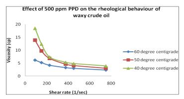
Figure 3: Effect of 500 ppm Pour Point Depressant on the Rheological Behaviour of Waxy Crude Oil at Different Temperature
