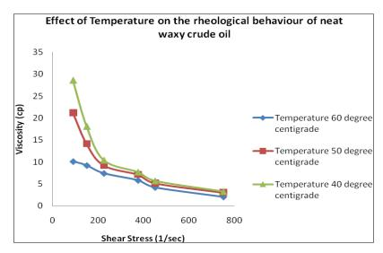
Figure 1: Effect of Temperature on the Rheological Behaviour of Neat Waxy Crude Oil
